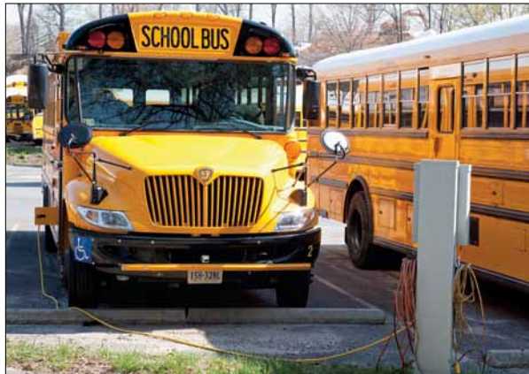
Charging the Hybrid Battery Pack
